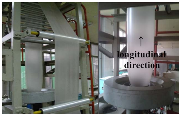
Figure 1. Continuous and stable preparation of starch/PVA nanocomposite films. [Color figure can be viewed in the online issue, which is available at wileyonlinelibrary.com .]
